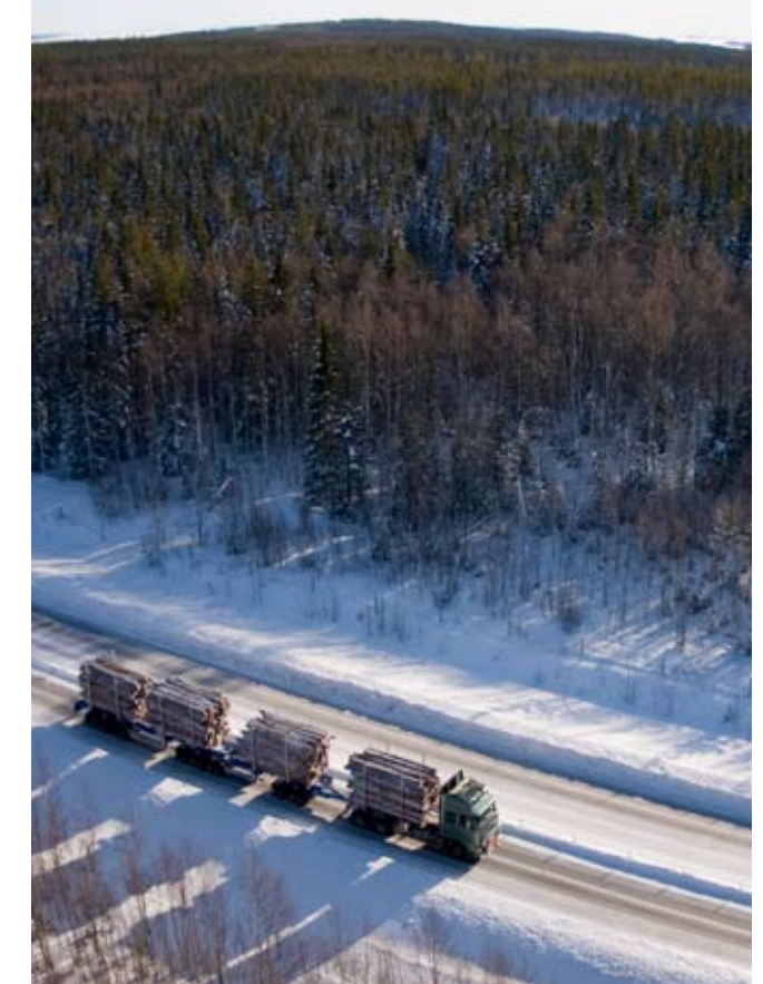
Sweden's longest timber load! The prototype vehicle produced within the framework of the ETT project (One more stack), will reduce carbon dioxide emissions by 23 percent compared to a conventional Swedish 60 ton timber vehicle. Photo: Erik Viklund
